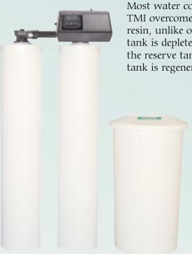
Most water conditioners deliver hard water during regeneration. 9100SXT TMI overcomes this problem by using two tanks containing ion exchange resin, unlike ordinary conditioners which use only one. As the capacity of one tank is depleted, the control valve automatically diverts the water supply to the reserve tank and conditioned water service is maintained. The depleted tank is regenerated and becomes the reserve.
